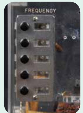
Close-up of the five black buttons used to create tones for the music box.
