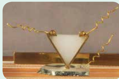
A simplified model of Bardeen and Brattain's original transistor of December 1947. Covering the edge of a plastic triangle with gold foil, then cutting a slit 2/1000 of an inch in the foil at the point of the triangle and placing both pieces into contact with a block of germanium, the scientists created the first transistor.
