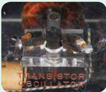
The box's "Transistor Oscillator." This is one of the early Type-A, point-contact transistors developed by William Pfann, the first practical transistor. The transistor acted as an oscillator when the black buttons were pushed and amplified the sound as it moved to the speaker.
