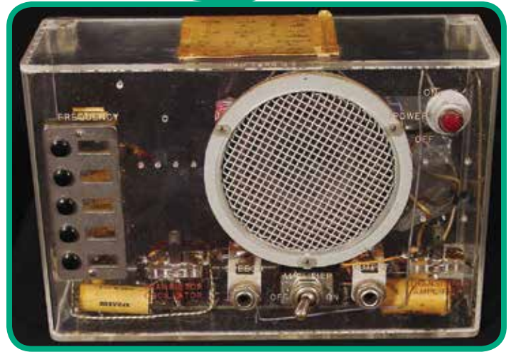
General view of the front of the music box. The interior is visible through the clear plastic case. On the left are the buttons which made the musical tones. On each side of the round speaker are the two transistors, marked as "Transistor Oscillator" on the left and "Transistor Amplifier" on the right. 1991.04.0110.
