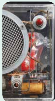
The right side of the music box, showing the "transistor amplifier" that was used when the box was connected to an external speaker. To the left of the transistor is the plug for connecting the speaker. The red button on the upper right is the power switch.
